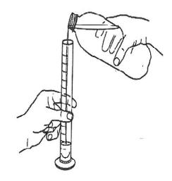
b. Observe and record the volume of water. The surface of the water will be curved in the cylinder. Read the volume at the bottom of this curve.
