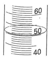
c. Carefully place the object you are measuring into the cylinder. It must be completely submerged.
